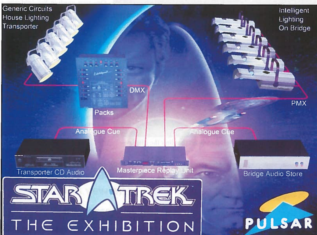
Pulsar's graphic shows how the Replay Unit controls lights, Dyalite dimmers and audio equipment.
